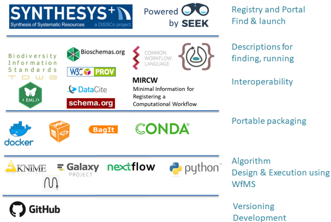
Image 3: The recommended workflow technology stack for the SDR
